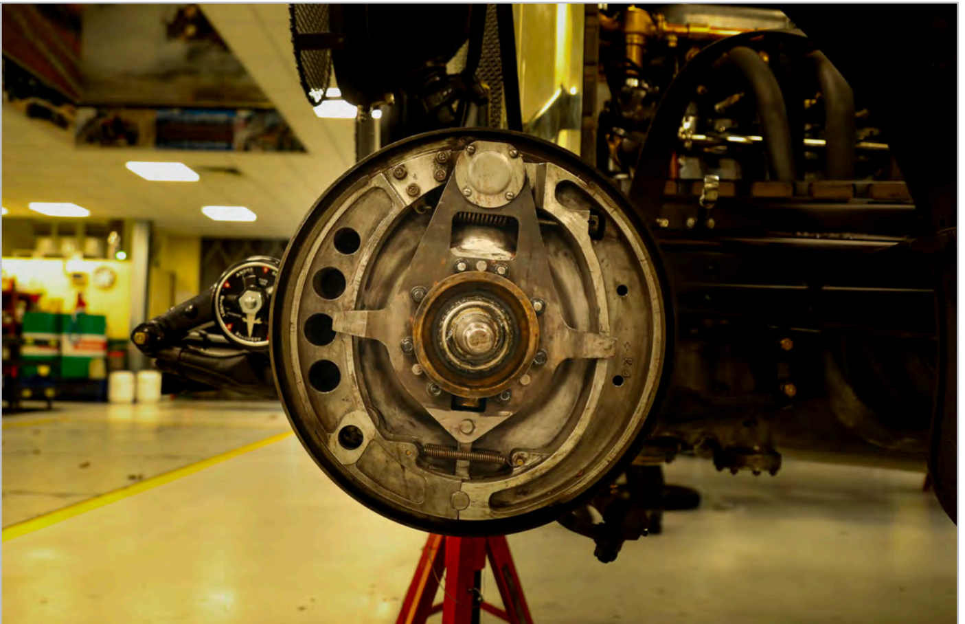
Front Axle Assembly - Self Wrapping Brakes 202719
