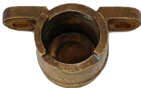
Cone Clutch Pedal Shaft Mounting Bracket N/S 202722
