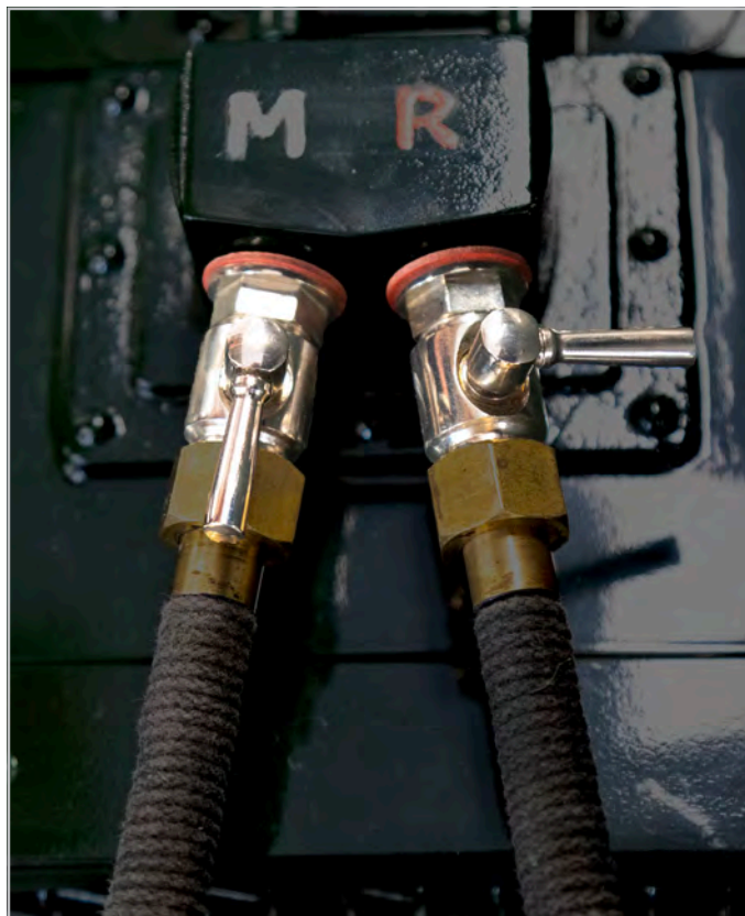
Air/Fuel Isolator Tap Brass: 200046 Chrome: 200121 Nickel: 202835
